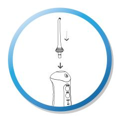
Insert the jet tip into the spray head hole until you hear a "click"
