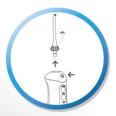
When removing or replacing the irrigator tip, please press the release button on the handle of the irrigator tip before removing it.
